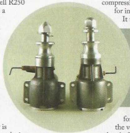
Parra T3 (right) shares principal dimensions and design elements with the Oliver Tiger Mk 3 engine (left). Note the T3's prop diver, which cups over the crankcase nose to protect front bearing from dirt.
