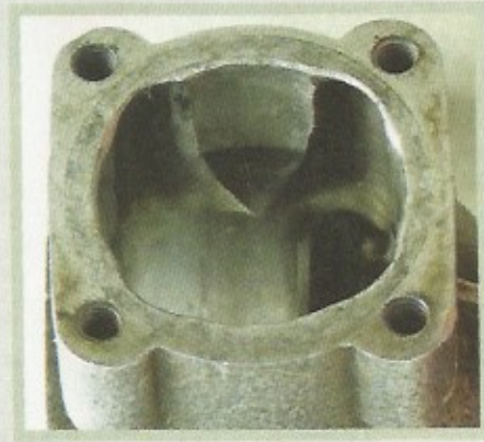
Close up shot of factory modified Oliver Tiger Mk 3 crankcase. Note the flared lower transfer passages aimed at improving gas flow.
