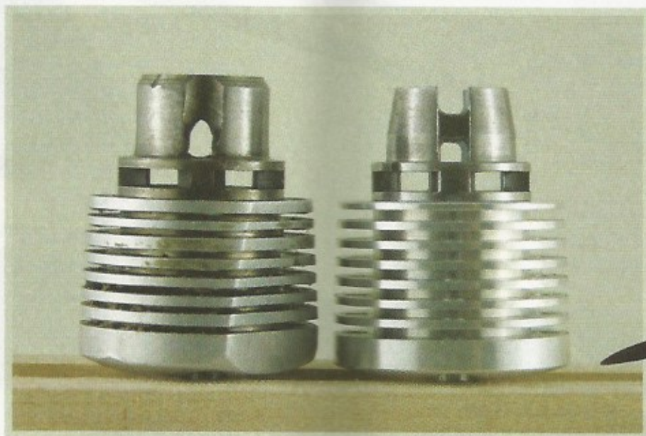
Oliver Tiger (L) and Parra T3 (R) cylinder assemblies have significant exterior differences, but actual port openings in the cylinder bore are almost identical.
