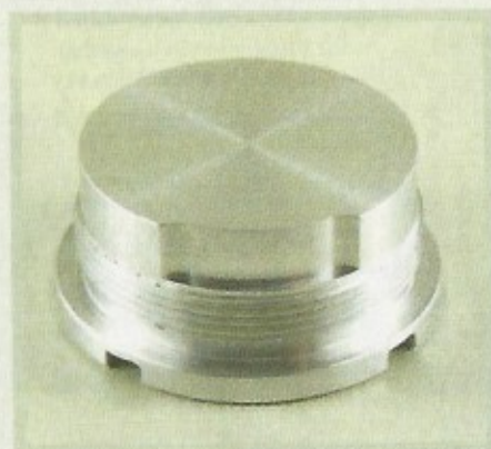
People who don't read instructions, beware! Backplate recess clears piston at bottom dead centre. Piston must be moved upwards out of the way when backplate is removed, or it'll end in tears.
