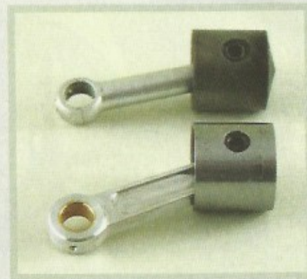
Oliver piston/conrod (top) compared with Parra assembly. Upper 2.5mm of piston diameter is reduced by 0.03mm (0.001 in.) a standard feature of modern high performance engines.
