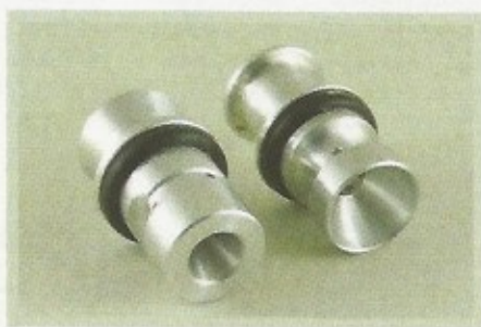
New venturi insert design (L) has fewer jets, smaller fuel channel and downstream aperture volumes when compared with earlier design (R). It provides more consistent running.
