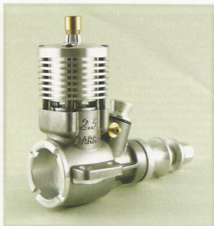
T3 has Parra's usual four-slot back plate. Crankcase is intricately relieved between the two high quality ball races, providing a very limber bottom end assembly.
